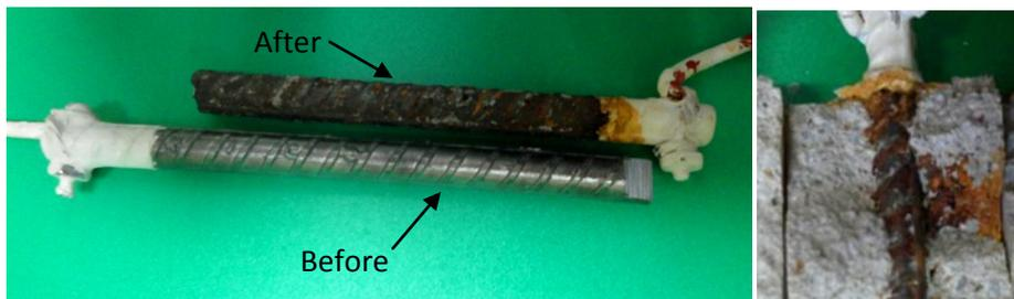
Figura 7. Reinforcing Steel after ACTIV.
