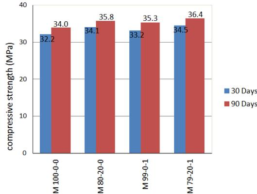
Figure 5. compressive strenght of hardened mortar.
